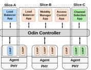
Figure 4: Odin applications operate upon a view of LVAPs and physical APs in their respective slices.
