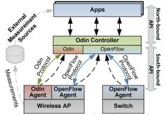
Figure 1: High-level design of the Odin architecture.
