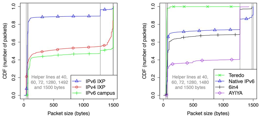
(a) Packet size distributions of IPv4 and IPv6 traffic (IXP and campus).
