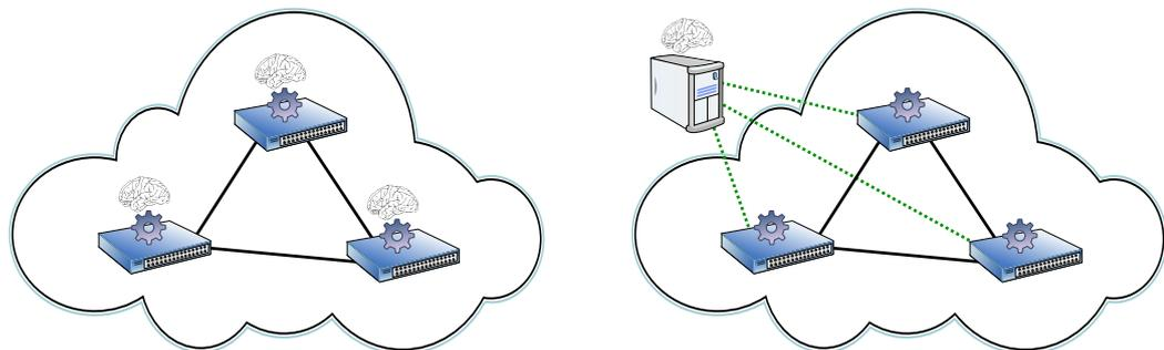
(a) A common network consisting of three routers or switches.
