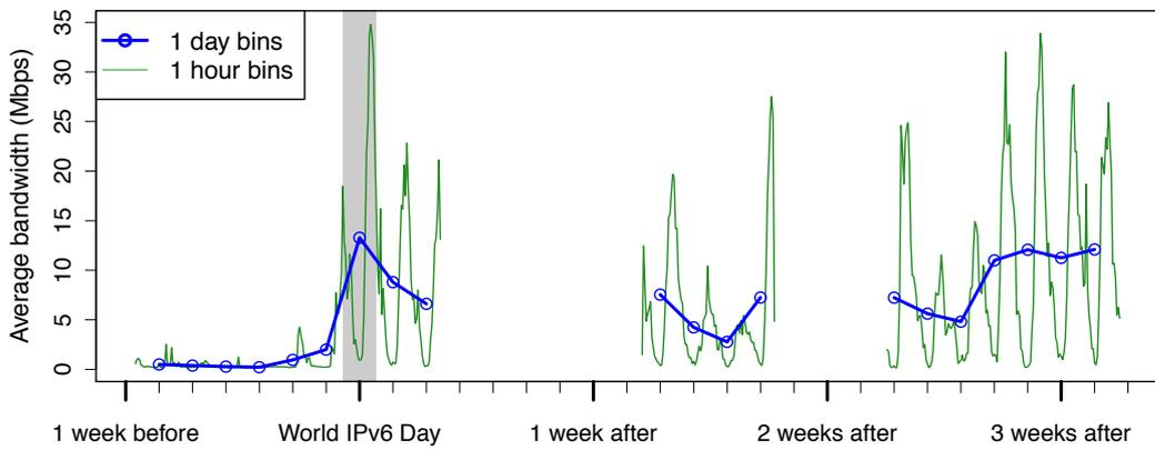
**Figure 8.2:** Total IPv6 traffic volume over time (campus). The tick marks are at noon UTC.
