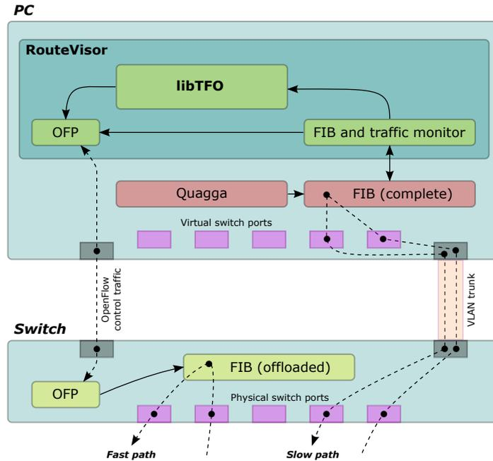
**Figure 3.2:** SDN Router prototype implementation based on a Linux PC running Quagga and RouteVisor (top), and an OpenFlow-enabled switch (bottom).
