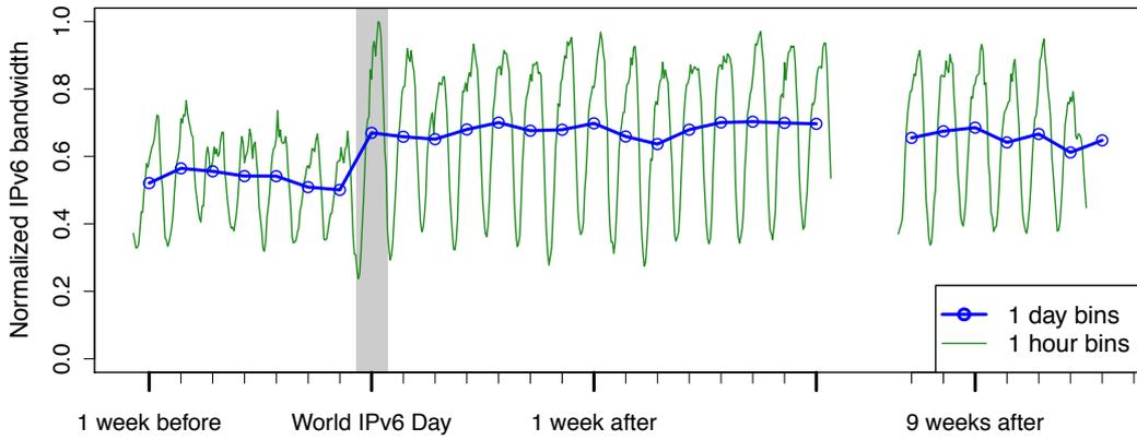
**Figure 8.1:** Total IPv6 traffic volume over time (IXP). The tick marks are at noon UTC.
