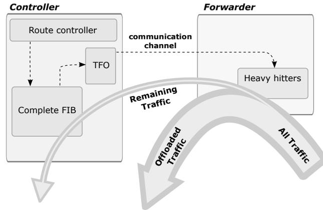
Figure 4.1: Traffic offloading system principle.
