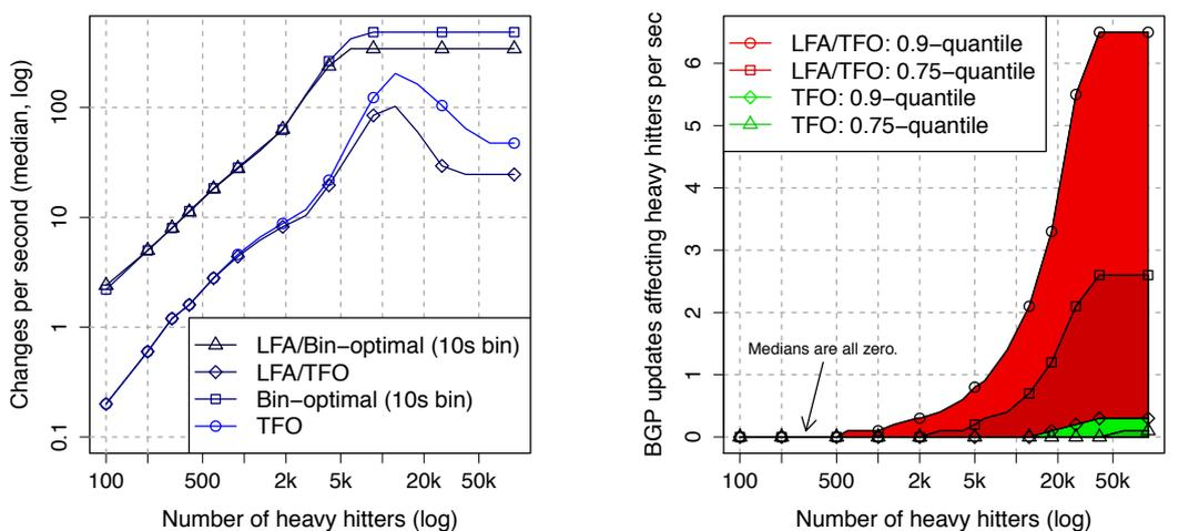
(a) Traffic offloading churn in the heavy hitters.
