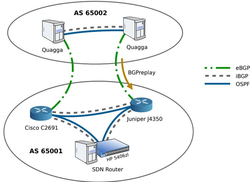
**Figure 3.3:** SDN Router interoperability test network topology.
