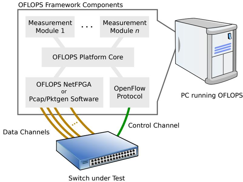
**Figure 6.1:** OFLOPS design schematic.
