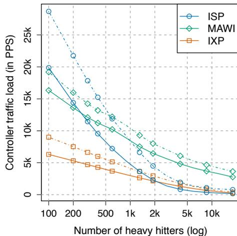
**Figure 4.9:** Controller traffic load under TFO (all traces).
