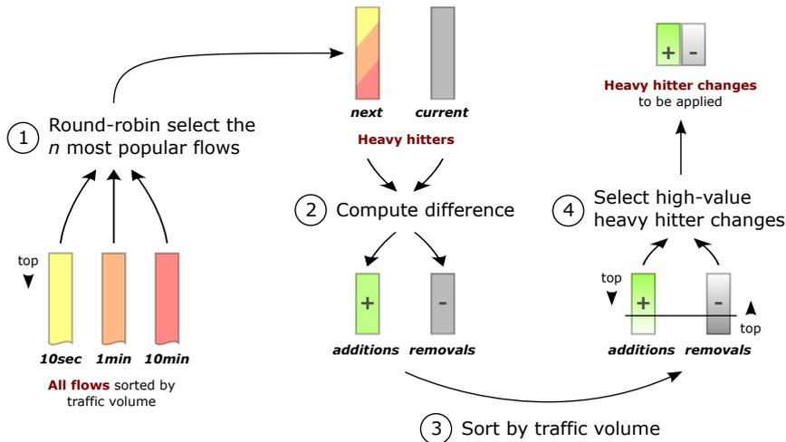
**Figure 4.7:** Functional diagram of Traffic-aware Flow Offloading (TFO).
