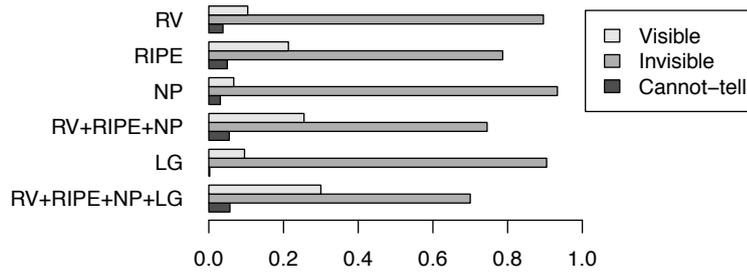
**Figure 7.3:** Peering links and visibility in control/data plane (normalized by number of detected P-P links).
