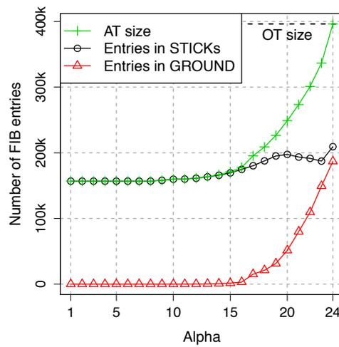
**Figure 5.5:** Size of aggregated STICKs and GROUND as a function of  $\alpha$ .
