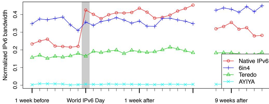
**Figure 8.3:** IPv6 traffic volume by tunnel encapsulation (IXP).
