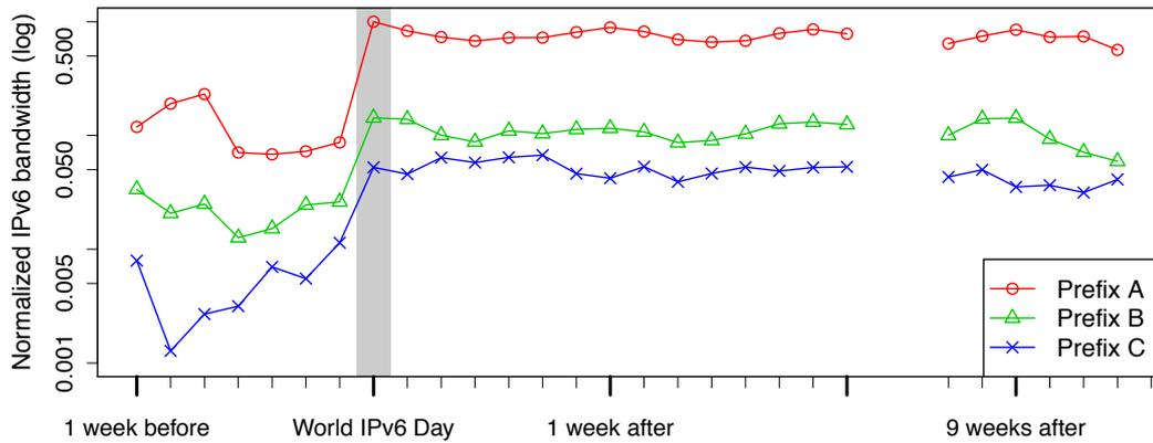
**Figure 8.8:** Normalized bandwidth of *all* IPv6 traffic per prefix before, at, and post the World IPv6 Day (IXP). The plot shows three examples out of the top ten high-volume IPv6 prefixes. Note the log-scale y-axis.
