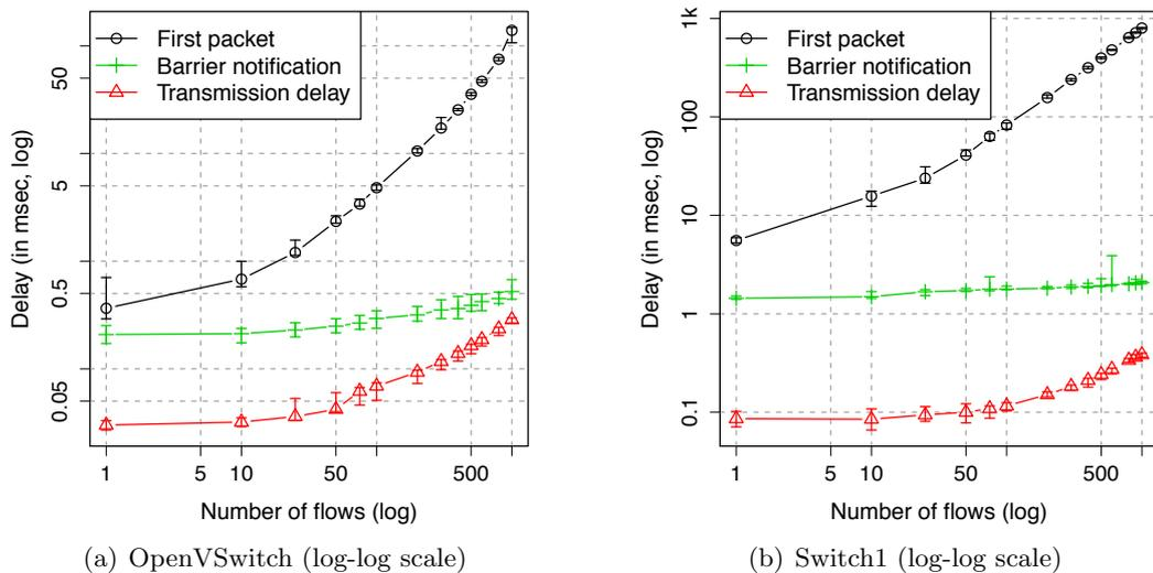
**Figure 6.3:** Flow entry insertion delay as obtained by using the `barrier` notification and as observed at the data plane.
