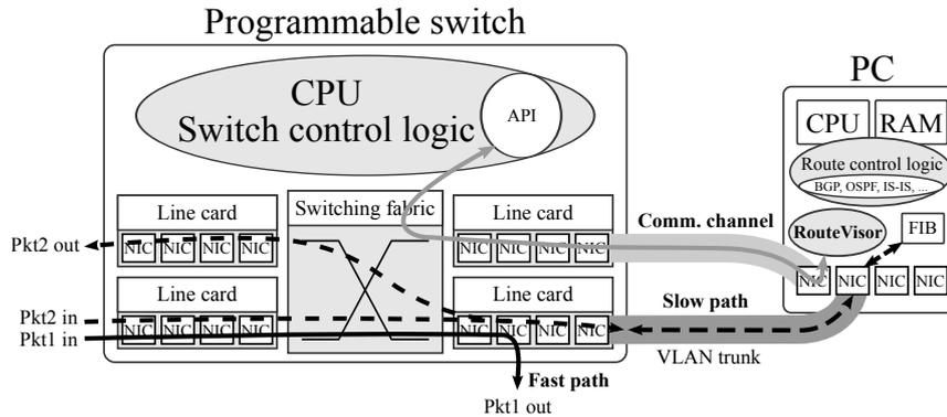
**Figure 3.1:** SDN Router concept with slow path (dashed black arrow), fast path (solid black arrow), and communication channel (grey arrow).
