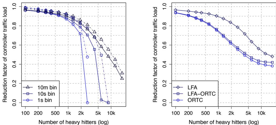
(a) Impact of LFA on controller load under bin-optimal. Dotted curves represent max values.
